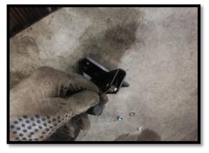
5. Wear the washer on the Ø6x35mm bolt and then pass it through the hitch apertures.
